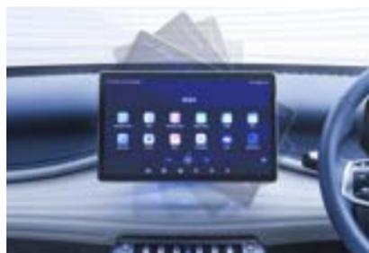
12.8-inch (32.5cm) Adaptive Rotating Suspension Electronic Pad
