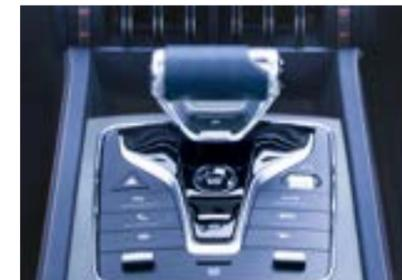
Push-type Electronic Gear Lever
